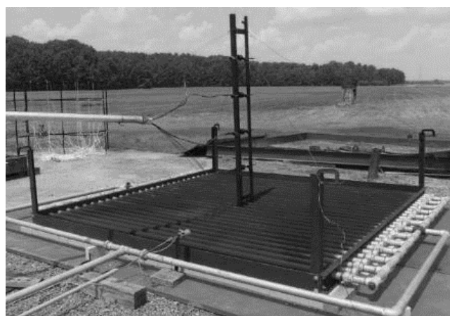
Figure A-3: Vertical rake for heat flux measurements.
